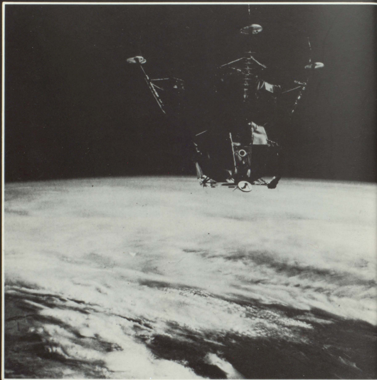
A view of the Lunar Module (LEM) photographed during its earth-orbital mission. The "Spider" is flying upside down in relation to the earth below. The landing gear on the LEM has been deployed and lunar surface probes (sensors) extend out from the landing gear foot pad.
